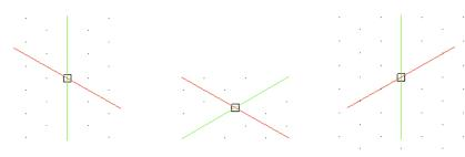
Notice the isometric cursor with its slanted cross hairs. It tells you which isometric drawing plane is current. There are three planes: left, top, and right (or front).
